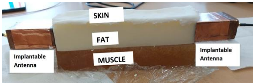
A radio link from two Fat-IBC matched antennas through a skin-fat-muscle planar phantom model
