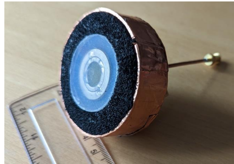
Perspective view of the shielded antenna. The antenna itself measures ~24 mm in diameter.
