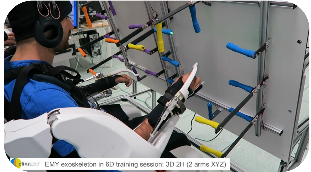
3D continuous trajectories and pronation/supination control of 2 arms 8D multi-limbs control
